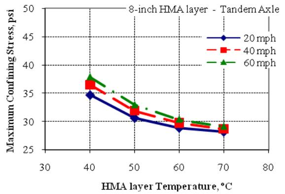
Figure E2c.2. Maximum deviator and confining stresses at 2-inch below the pavement surface of the PG52-22 mix
