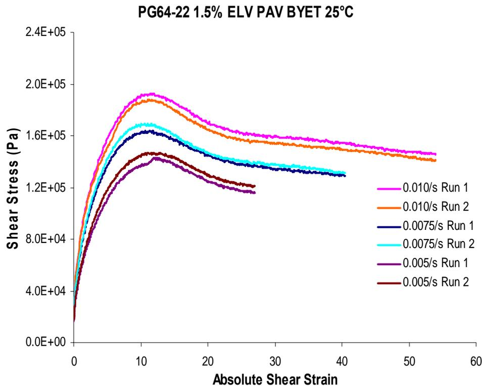
Figure F2e.1. Graph. BYET results for an ELV-modified PG 64-22 base binder at 25 °C.
