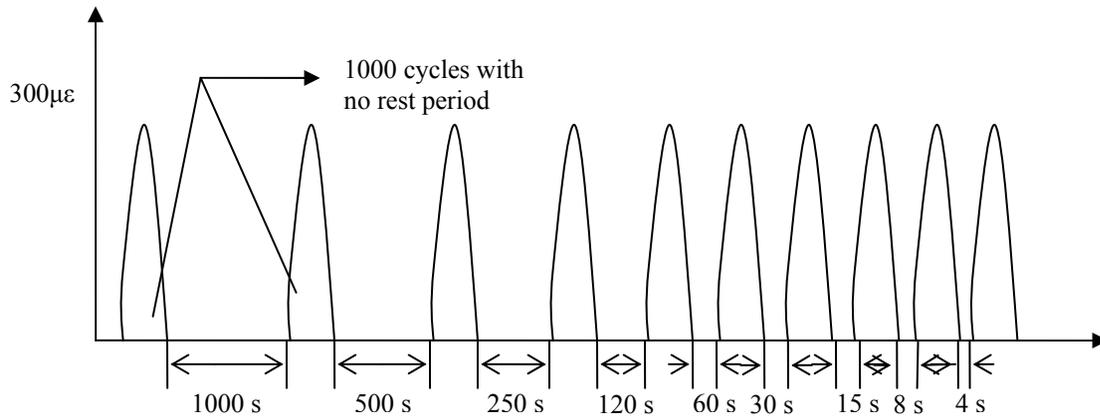
Figure F2c.1 Loading configuration for revised RDT test.
