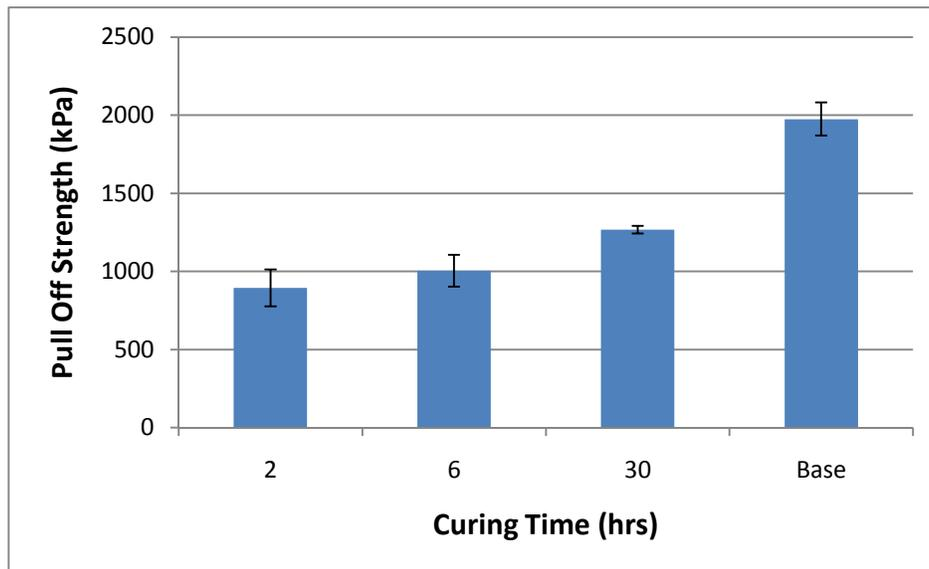
Figure E1c-2.4. Graph. Adhesion testing results for CRS-2 emulsion after 2-, 6- and 30-hour curing times.
