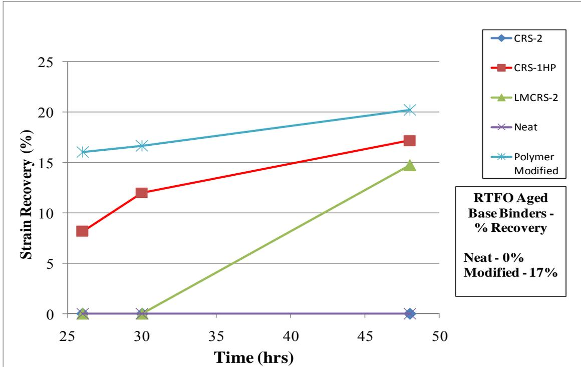
Figure E1c-2.1. Graph. Percent strain recovery for different emulsions as a function of residue recovery time.
