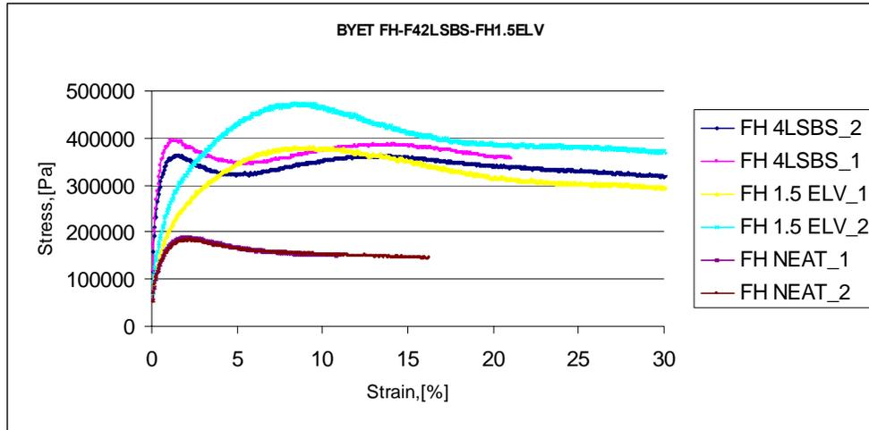
Figure F2a.1. Graph. Stress versus strain for FH-based binder.
