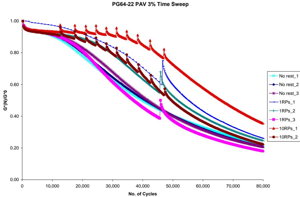
Figure F1d-6.1. Graph. Fatigue damage plots for PG 64-22.
