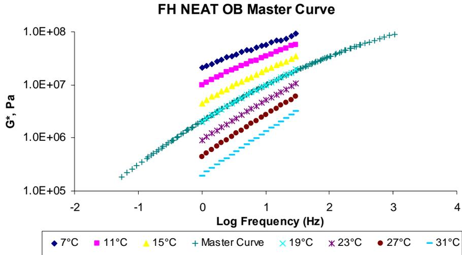
Figure F2a.3. Graph. Master curve FH original binder.
