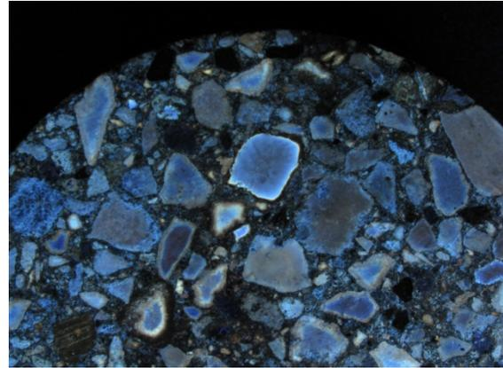
(b) Asphalt Mixture under Ultraviolet Light
