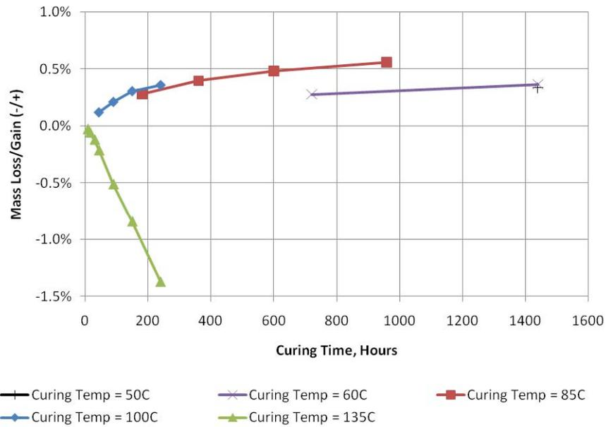
Figure E2d.2. PG64-22 Mass loss/gain at various curing temperatures and times.
