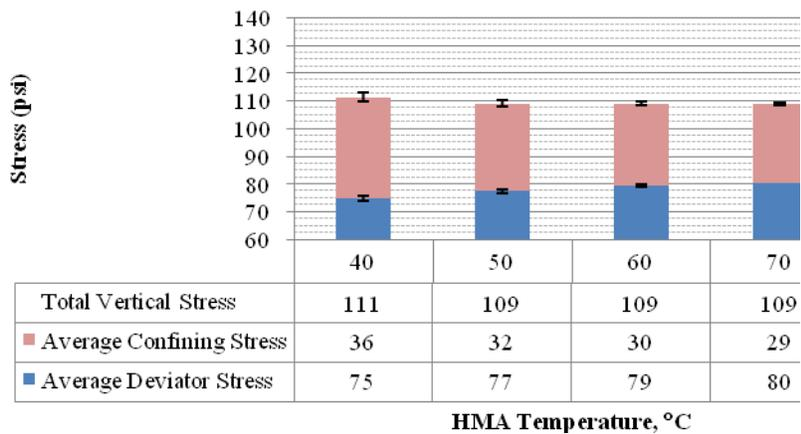
Figure E2c.4. Average Maximum deviator, confining, and total stresses of the various pavement structures – PG52-22 mix
