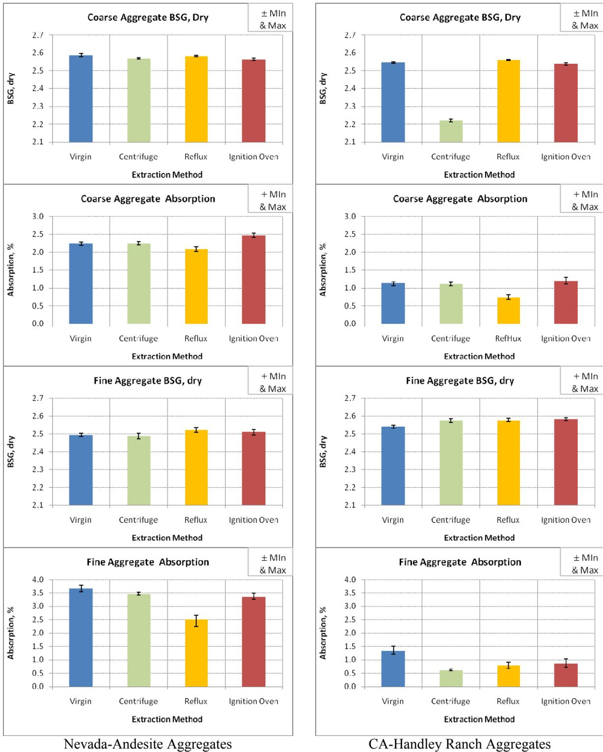
Figure E2b.2 Specific gravity and absorption of fine and coarse aggregates (AASHTO T84 and AASHTO T85)
