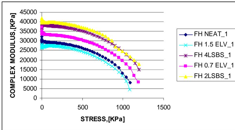
Figure F2a.2. Graph. Complex modulus versus stress for FH-based binder.
