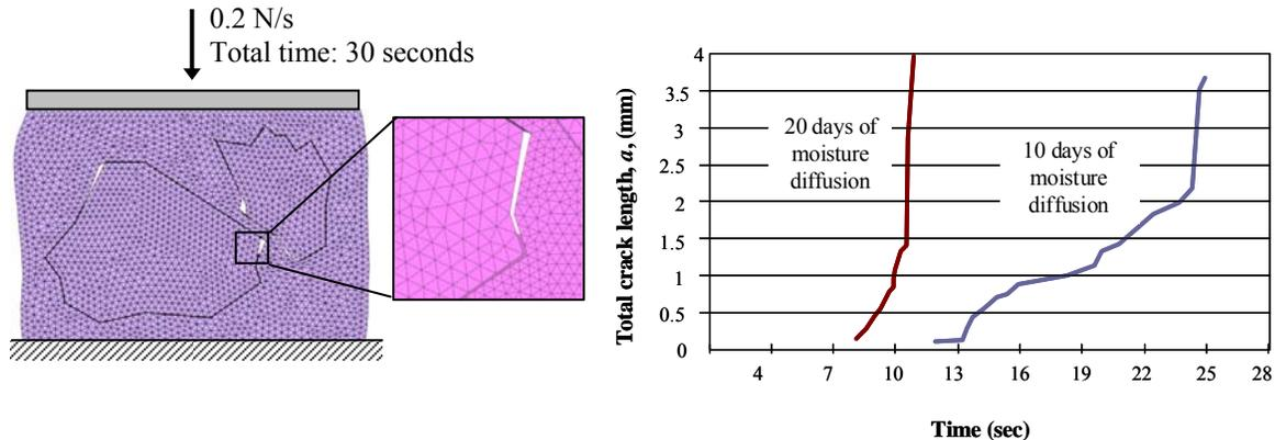
Figure M4a.2. Crack length at the interface vs. time during the mechanical test conducted on a sample subjected to 20 days of moisture diffusion and a sample subjected to 10 days of moisture diffusion (same boundary conditions).
