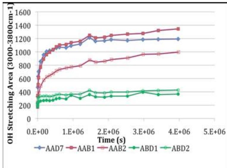
Figure M2b.1. Typical results for moisture diffusion through thin films of asphalt binders as recorded using the FTIR
