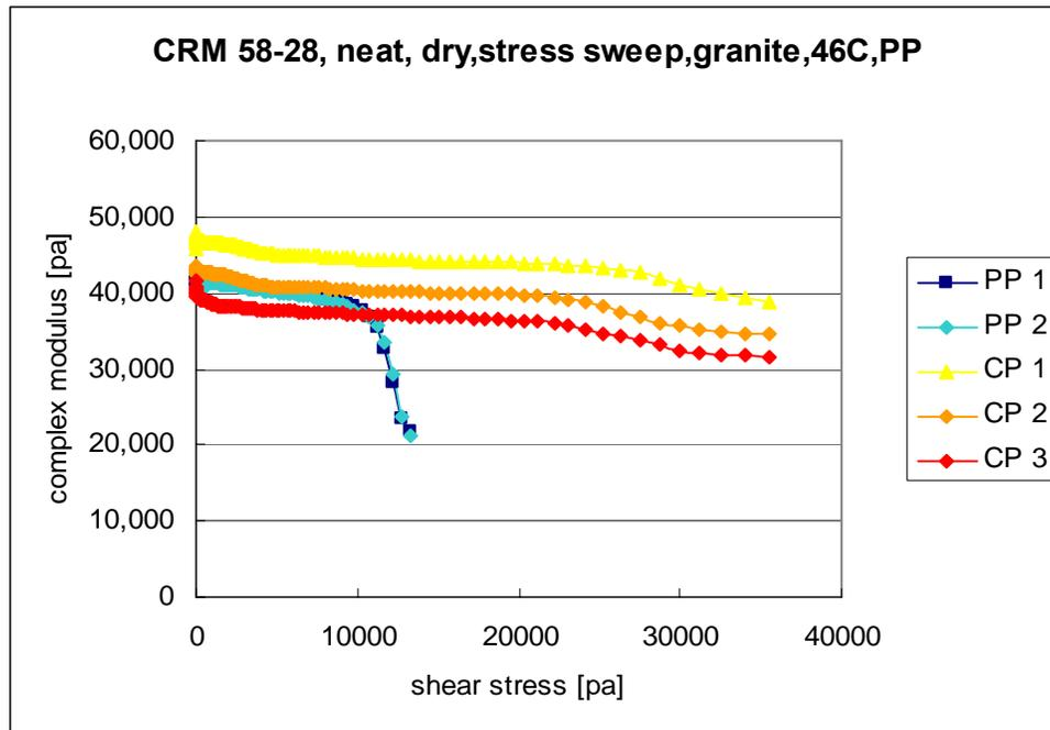
Figure M1a.3. Graph. Stress sweep testing results at 46 °C for the CRM neat binder in dry conditions, with granite and with cone-and-plate and parallel-plate.
