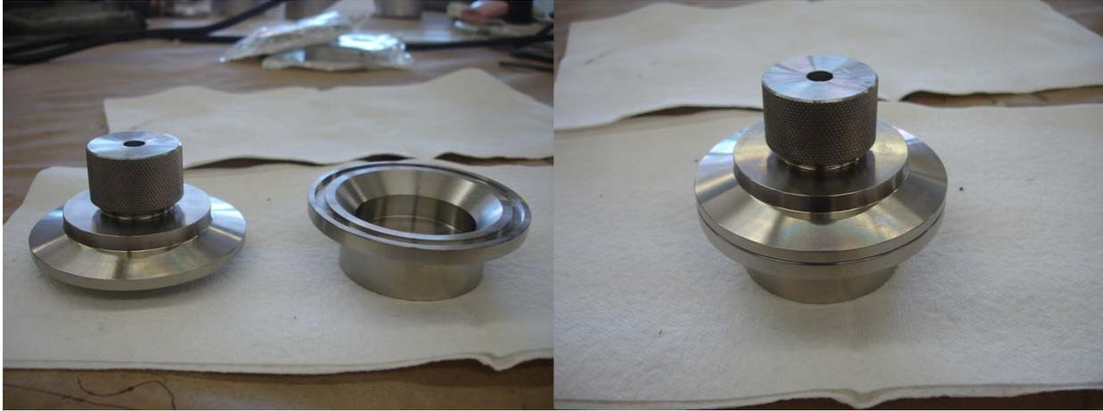
Figure E2d.1. New cell prototype for the glass transition temperature measurement equipment.
