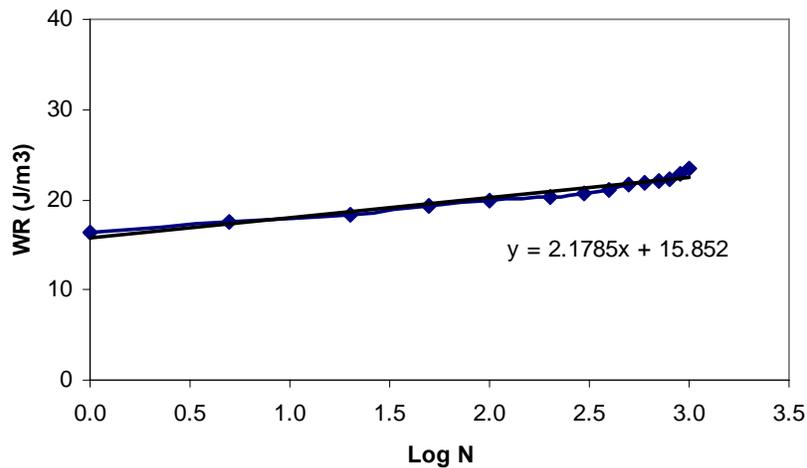
Figure F2c.2 Relationship between DPSE and number of load cycles.
