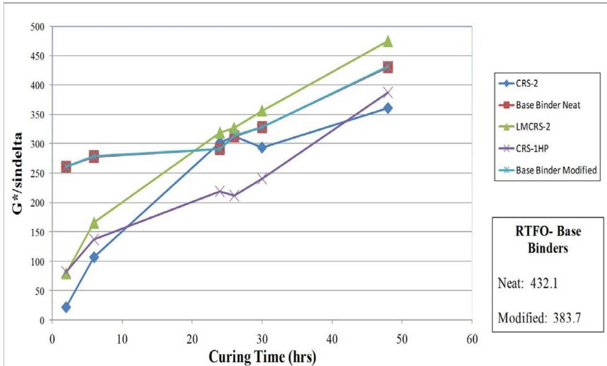
Figure E1c-2.2. Graph.  $G^*/\sin(\delta)$  of the emulsion residue as a function of recovery time.
