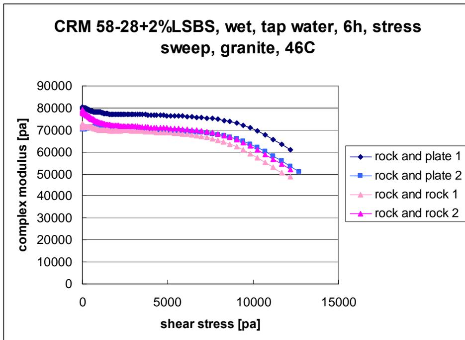
Figure M1a.2. Graph. Stress sweep testing results at 46 °C for the CRM modified with 2% wt linear styrene-butadiene-styrene (LSBS) binder in wet conditions, after 6 hours conditioning in tap water, with granite rock disks.
