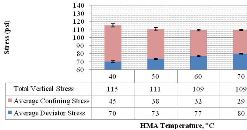
Figure E2c.3. Average Maximum deviator, confining, and total stresses of the various pavement structures - PG64-22 mix
