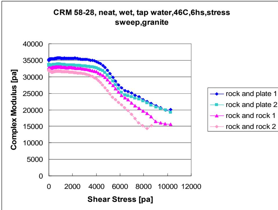
Figure M1a.1. Graph. Stress sweep testing results at 46 °C for the CRM neat binder in wet conditions, on granite after 6 hours conditioning in tap water.
