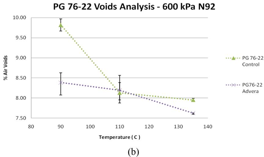
Figure E1c-1.2. Graphs. Plots of percent air voids versus compaction temperature for (a) PG 64-22 and (b) PG 76-22 mixtures.
