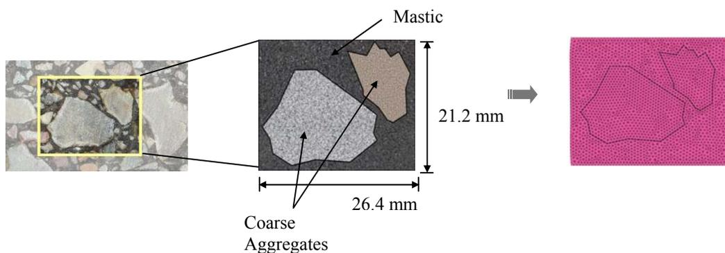
Figure M4a.1. Geometry and finite element implementation of a micromechanical model from a real asphalt mixture.
