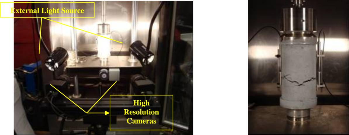
Figure F3b-1.2. Digital Image correlation (DIC) testing system and a specimen after testing.
