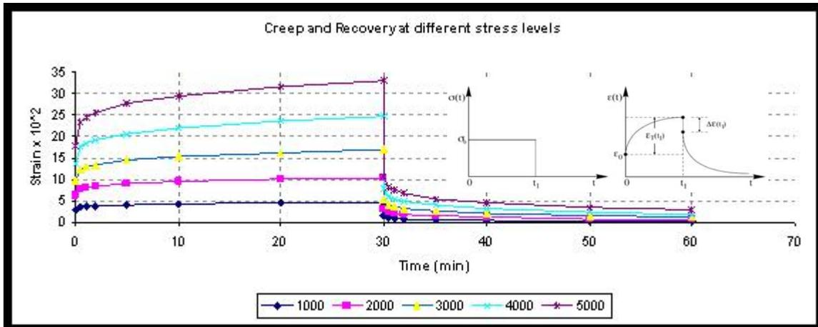
Figure F1b.1. Sample creep-recovery data used to obtain the four non-linear parameters following the approach developed by Schapery.
