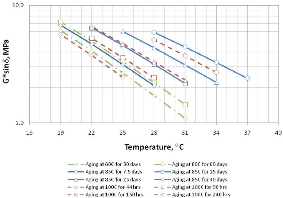
Figure E2d.3.  $G^* \sin \delta$  for the PG64-22 at various temperatures and curing times.
