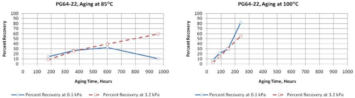
Figure E2d.4. Percent recovery of the PG64-22 asphalt binder from the MSCR test.
