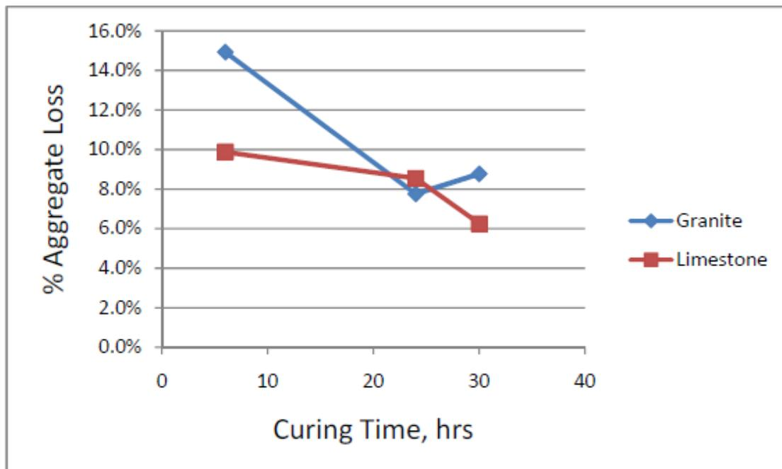
Figure E1c-2.3. Graph. Percent aggregate retention as a function of time for granite and limestone chips applied to a CRS-1HP emulsion.
