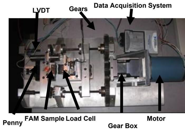
(a) Configuration of the fracture testing system
