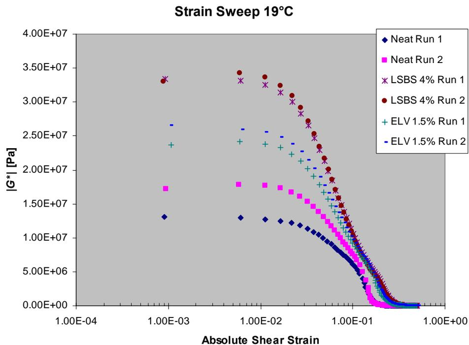
Figure F2e.2. Graph. Strain sweep results for three materials at 19 °C (unmodified base binder, binder modified with 4% LSBS and binder modified with 1.5% ELV).
