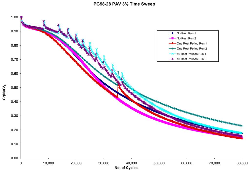
Figure F1d-6.2. Graph. Fatigue damage plots for PG 58-28.
