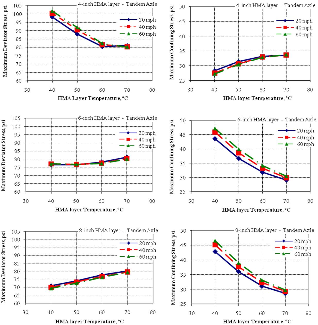
Figure E2c.1. Maximum deviator and confining stresses at 2-inch below the pavement surface of the PG64-22 mix
