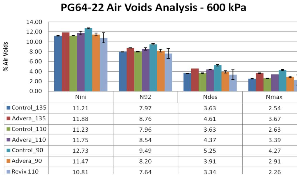
Figure E1c-1.1. Graph. Plot of air voids analysis for mixtures using PG 64-22 binder at 600 kPa compaction pressure.
