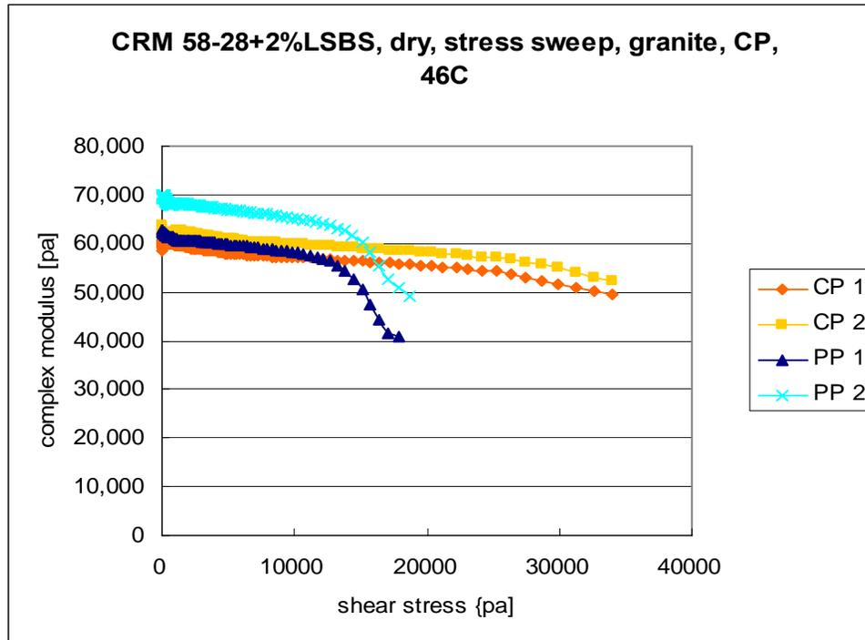
Figure M1a.4. Graph. Stress sweep testing results at 46 °C for the CRM modified with 2% wt LSBS binder in dry conditions, with granite and with cone-and-plate and parallel-plate. (CP = cone-and-plate, PP = parallel-plate)
