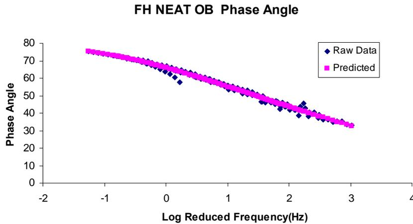
Figure F2a.4. Graph. Phase angle versus frequency FH original binder.
